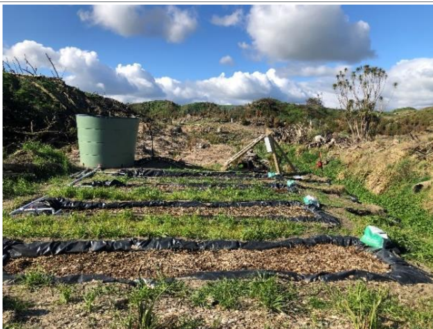
Four small scale bio-reactor installations at the POT for research experimental purpose.
